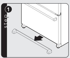
Remove toe grille. Grasp firmly and pull outward
